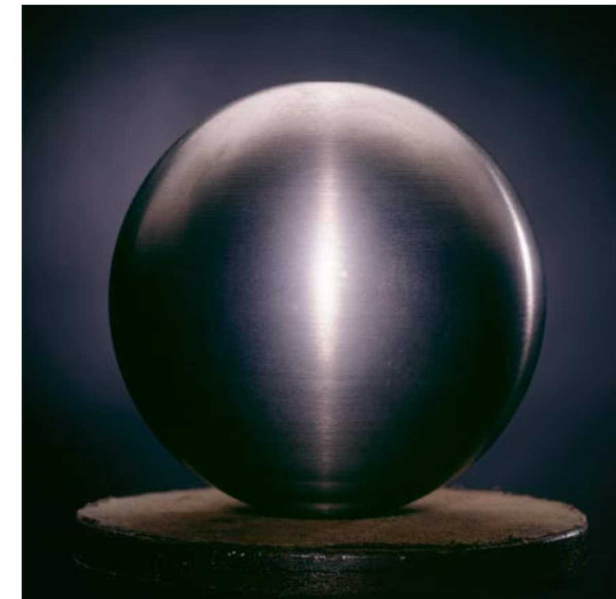
Tungsten pendulum weights, machined to 1/10,000th of an inch just part of the intricate mechanism of the Clock of the Long Now.
