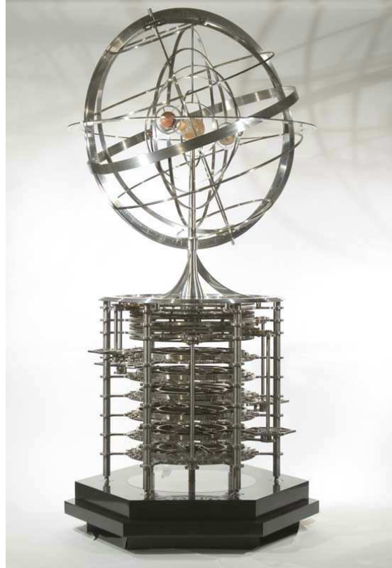
Figure 7. Prototype of the 10,000-Year Clock's Copernican orrery, currently on display at the Long Now Foundation's museum in San Francisco, CA
