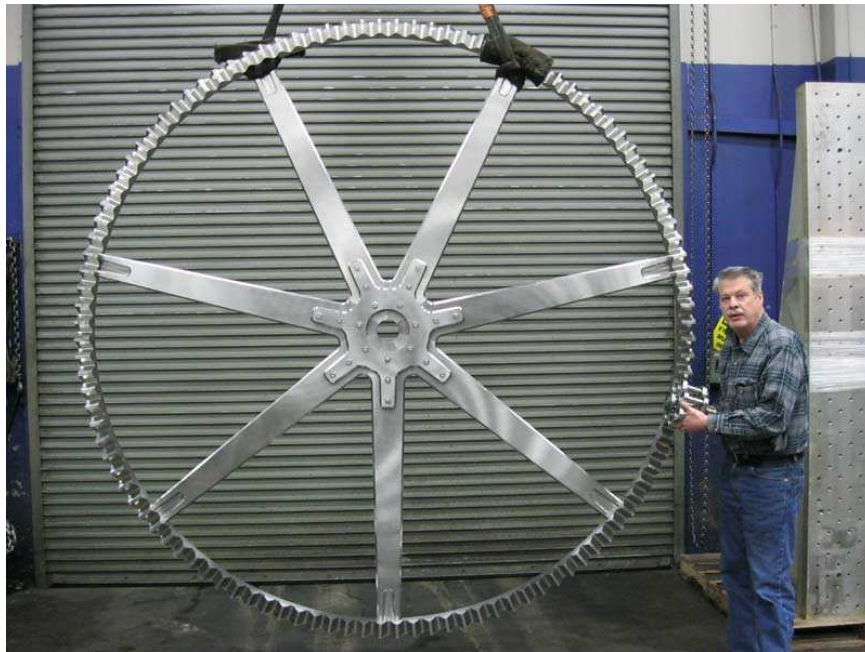
Figure 1. A drive gear to be used in the 10,000-year clock.
